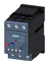
Overload relay 22...32 A Thermal For motor protection Size S2, Class 10 Stand-alone installation Main circuit: Screw Auxiliary circuit: Screw Manual-Automatic-Reset
