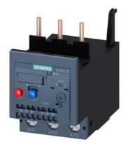
Overload relay 22...32 A Thermal For motor protection Size S2, Class 10 Contactor mounting Main circuit: Screw Auxiliary circuit: spring-type terminal Manual-Automatic-Reset
