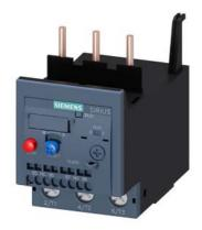
Overload relay 40... 50 A Thermal For motor protection Size S2, Class 10 Contactor mounting Main circuit: Screw Auxiliary circuit: spring-type terminal Manual-Automatic-Reset
