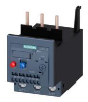
Overload relay 47...57 A Thermal For motor protection Size S2, Class 10 Contactor mounting Main circuit: Screw Auxiliary circuit: spring-type terminal Manual-Automatic-Reset
