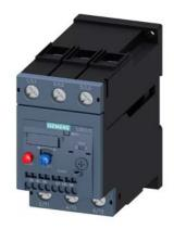
Overload relay 47...57 A Thermal For motor protection Size S2, Class 10 Stand-alone installation Main circuit: Screw Auxiliary circuit: spring-type terminal Manual-Automatic-Reset
