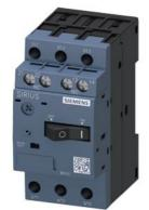
Circuit breaker size S00 for motor protection, CLASS 10 A-release 0.55...0.8 A N-release 10 A Screw terminal Standard switching capacity with transverse auxiliary switch 1 NO+1 NC  $\,$
