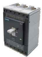
Molded case circuit breaker 3RV1 for motor protection Standard switching capacity Rated current In = 400 A electronic release Short-circuit protection adjustable 6-13 x In Overload protection adjustable 0.4-1 x In, Class 10A-33 Icu = 120 kA at 400 V 3-pole, Screw terminal including phase barriers
