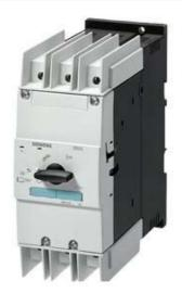
CIRCUIT-BREAKER, SIZE S3, FOR THE PLANT PROTECTION, WITH APPROBATION CIRC.-BREAKER UL 489, CSA C22.2 NO.5-02, A-TRIGGER 10 A, N-TRIGGER 150 A, SCREW CONNECTION, STANDARD SWITCHING CAPACITY
