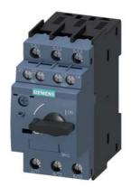
Circuit breaker size S0 for motor protection, CLASS 10 A-release 0.45...0.63 A N-release 8.2 A screw terminal Standard switching capacity with transverse auxiliary switches 1 NO+1 NC
