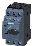
Circuit breaker size S0 for motor protection, CLASS 10 A-release 27...32 A N-release 400 A screw terminal Standard switching capacity with transverse auxiliary switches 1 NO+1 NC
