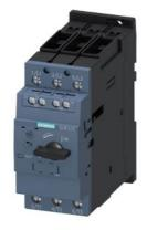
Circuit breaker size S2 for motor protection class 20 A-release 14...20 A N-release 260 A screw terminal Standard switching capacity with transverse auxiliary switch 1 NO+1 NC
