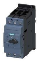
Circuit breaker size S2 for motor protection, Class 20 A-release 18...25 A N-release 325 A Screw terminal Standard switching capacity
