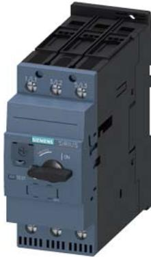
Circuit breaker size S2 for motor protection, Class 20 A-release 54...65 A N-release 845 A screw terminal Standard switching capacity
