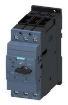
Circuit breaker size S2 for motor protection, Class 20 A-release 28...36 A N-release 520 A screw terminal Standard switching capacity
