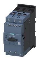
Circuit breaker size S3 for motor protection, CLASS 10 A-release 57...75 A N-release 975 A screw terminal Standard switching capacity with transverse auxiliary switches 1 NO+1 NC
