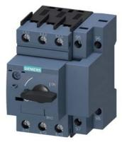
Circuit breaker size S00 for motor protection, CLASS 10 with overload relay function A-release 0.14...0.2 A N-release 2.6 A screw terminal Standard switching capacity
