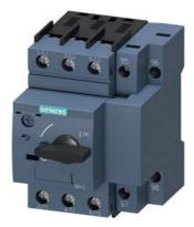
Circuit breaker size S00 for motor protection, CLASS 10 with overload relay function A-release 0.7...1 A N-release 13 A screw terminal Standard switching capacity
