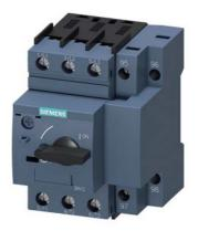
Circuit breaker size S00 for motor protection, CLASS 10 with overload relay function A-release 1.1...1.6 A N-release 21 A screw terminal Standard switching capacity
