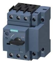
Circuit breaker size S00 for motor protection, CLASS 10 with overload relay function A-release 2.8...4 A N release 52 A screw terminal Standard switching capacity
