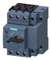
Circuit breaker size S00 for motor protection, CLASS 10 with overload relay function A-release 5.5...8 A N-release 104 A screw terminal Standard switching capacity
