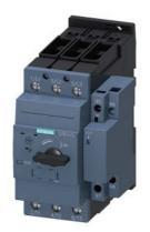
Circuit breaker size S2 for motor protection, CLASS 10 with overload relay function A-release 9.5...14 A N-release 208 A Standard switching capacity
