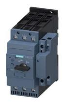
Circuit breaker size S2 for motor protection, CLASS 10 with overload relay function A-release 42...52 A N-release 741 A Standard switching capacity
