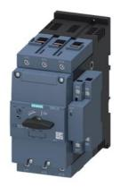
Circuit breaker size S3 for motor protection CLASS 10 with overload relay function A-release 75...93 A N-release 1300 A screw terminal Increased switching capacity 100 kA  $\,$
