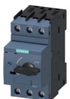
Circuit breaker size S00 for starter combination Rated current 0.16 A N-release 2.1 A screw terminal Standard switching capacity
