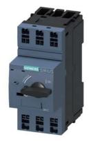
Circuit breaker size S00 for starter combination Rated current 2 A N-release 26 A Spring-type terminal Standard switching capacity
