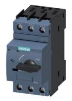
Circuit breaker size S0 for starter combination Rated current 4 A N release 52 A screw terminal Standard switching capacity
