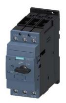
Circuit breaker size S2 for starter combination Rated current 14 A N-release 208 A screw terminal Standard switching capacity
