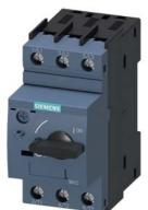
Circuit breaker size S00 for transformer protection A-release 10...16 A N-release 286 A screw terminal Standard switching capacity
