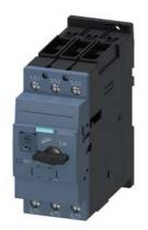
Circuit breaker size S2 for transformer protection A-release 32...40 A N-release 820 A screw terminal Standard switching capacity
