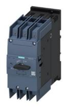
Circuit breaker size S3 for system protection with approval circuit breaker UL 489, CSA C22.2 No.5-02 A-release 35 A N-release 455 A screw terminal
