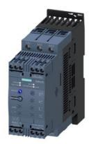
SIRIUS soft starter S2 72 A, 37 kW/400 V, 40  $^{\circ}\text{C}$  200-480 V AC, 24 V AC/DC Screw terminals Thermistor motor protection
