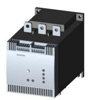
SIRIUS soft starter S12 230 A, 160 kW/500 V, 40 °C 400-600 V AC, 230 V AC Screw terminals !!! Phased-out product !!! Successor is SIRIUS 3RW5, Preferred successor type is >>3RW5073-6AB15<<
