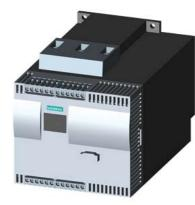
SIRIUS soft starter Values at 575 V, 50 °C standard: 26 A, 20 hp Inside-delta: 45 A, 40 hp 400-600 V AC, 115 V AC Screw terminals !!! Phased-out product !!! Successor is SIRIUS 3RW5, Preferred successor type is >>3RW5516-1HA15<<
