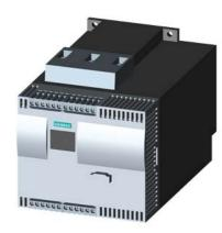
SIRIUS soft starter Values at 500 V, 40 °C standard: 57 A, 37 kW Inside-delta: 99 A, 55 kW 400-600 V AC, 230 V AC Screw terminals !!! Phased-out product !!! Successor is SIRIUS 3RW5, Preferred successor type is >>3RW5525-1HA16<<
