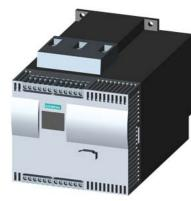
SIRIUS soft starter Values at 460 V, 50 °C standard: 68 A, 50 hp Inside-delta: 118 A, 75 hp 200-460 V AC, 115 V AC Screw terminals !!! Phased-out product !!! Successor is SIRIUS 3RW5, Preferred successor type is >>3RW5526-1HA14<<
