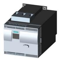
SIRIUS soft starter Values at 575 V, 50 °C standard: 68 A, 50 hp Inside-delta: 118 A, 100 hp 400-600 V AC, 115 V AC Screw terminals !!! Phased-out product !!! Successor is SIRIUS 3RW5, Preferred successor type is >>3RW5526-1HA16<<
