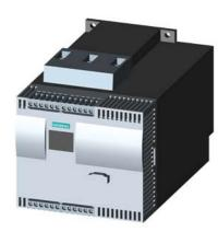
SIRIUS soft starter Values at 460 V, 50 °C standard: 82 A, 60 hp Inside-delta: 142 A, 100 hp 200-460 V AC, 115 V AC Screw terminals !!! Phased-out product !!! Successor is SIRIUS 3RW5, Preferred successor type is >>3RW5527-1HA14<<
