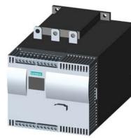
SIRIUS soft starter Values at 460 V, 50 °C standard: 100 A, 75 hp Inside-delta: 173 A, 125 hp 200-460 V AC, 115 V AC spring-type terminals !!! Phased-out product !!! Successor is SIRIUS 3RW5, Preferred successor type is >>3RW5534-2HA14<<
