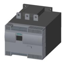
SIRIUS soft starter Values at 690 V, 40 °C standard: 203 A, 200 kW Inside-delta: only up to 600 V 400-690 V AC, 230 V AC spring-type terminals !!! Phased-out product !!! Successor is SIRIUS 3RW5, Preferred successor type is >>3RW5543-2HA16<<
