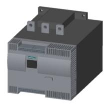
SIRIUS soft starter Values at 400 V, 40 °C standard: 432 A, 250 kW Inside-delta: 748 A, 400 kW 200-460 V AC, 230 V AC spring-type terminals !!! Phased-out product !!! Successor is SIRIUS 3RW5, Preferred successor type is >>3RW5547-2HA14<<
