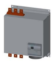
SIRIUS soft starter Values at 400 V, 40 °C standard: 615 A, 355 kW Inside-delta: 1065 A, 630 kW 200-460 V AC, 230 V AC Screw terminals !!! Phased-out product !!! Successor is SIRIUS 3RW5, Preferred successor type is >>3RW5552-6HA14<<
