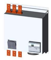
SIRIUS soft starter Values at 400 V, 40 °C standard: 1214 A, 710 kW Inside-delta: 2103 A, 1200 kW 200-460 V AC, 230 V AC Screw terminals !!! Phased-out product !!! Successor is SIRIUS 3RW5, Preferred successor type is >>3RW5558-6HA14<<
