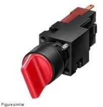
Selector switch, 16 mm, round, plastic, black, 3 switch positions I>O<II, momentary contact type, Retraction from left and right, Actuating angle 2 x 50 degree, 1 NO, 1 NO
