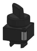
Selector switch, 22 mm, round, Plastic, Black, Selector switch, short, 3 switch positions I-O-II, Latching, Actuating angle 2x50 degrees, With holder !!! Phased-out product !!! Successor is SIRIUS ACT 3SU1 Preferred successor type is >>3SU1002-2BL10-0AA0 + 3SU1500-0AA10-0AA0<
