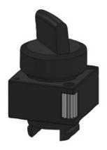
Selector switch, 22 mm, round, Plastic, Black, Selector switch, short, 3 switch positions I-O-II, Momentary contact type, Actuating angle 2x50 degrees, With holder !!! Phased-out product !!! Successor is SIRIUS ACT 3SU1 Preferred successor type is >>3SU1002-2BM10-0AA0+ 3SU1500-0AA10-0AA0<<
