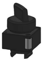
Selector switch, 22 mm, round, Plastic, Black, Selector switch, short, 3 switch positions I-O-II, Left latching, Right momentary contact type, Actuating angle 2x50 degrees, With holder !!! Phased-out product !!! Successor is SIRIUS ACT 3SU1 Preferred successor type is >>3SU1002-2BN10-0AA0 + 3SU1500-0AA10-0AA0<
