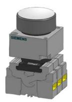
Illuminated pushbutton, 22 mm, round, plastic, blue, pushbutton, flat, with holder, 1 NO + 1 NO, Lampholder, with integrated LED 24 V AC/DC Screw terminal !!! Phased-out product !!! Successor is SIRIUS ACT 3SU1 Preferred successor type is >>3SU1102-0AB50-1FA0<<
