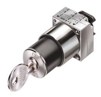
22MM METAL ROUND ACTUATOR: CES KEY-OPER.SWITCH WITH 2 KEYS MOMENTARY CONTACT TYPE 3 SWITCH POSITIONS I-O-II LOCK NO SSG 10, REMOVAL POS. O WITH HOLDER
