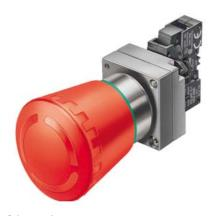
22MM METAL ROUND COMPLETE UNIT COMBINATION: EMERGEN.-STOP MUSHR.PUSHB. 40MM LATCH.W. ROT.-TO-UNLATCH MECH. WITH YELLOW BACKING PLATE SCREW TERMINAL, 1NC WITH HOLDER RED INSCRIPTION: NOT-HALT !!! Phased-out product !!! SIRIUS ACT 3SU1 is successor Preferred successor type is >>3SU1150-1HB20-1CH0<<
