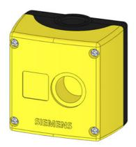
ENCLOSURE FOR COMMAND DEVICES, 22MM, ROUND, ENCLOSURE MATERIAL PLASTIC, ENCLOSURE TOP PART YELLOW, 1 COMMAND POINT, UNEQUIPPED, FLOOR MOUNTING, 1 X M20 EACH AT TOP AND BOTTOM !!! Phased-out product !!! SIRIUS ACT 3SU1 is successor Preferred successor type is >>3SU1801-0AA00-0AB2<<
